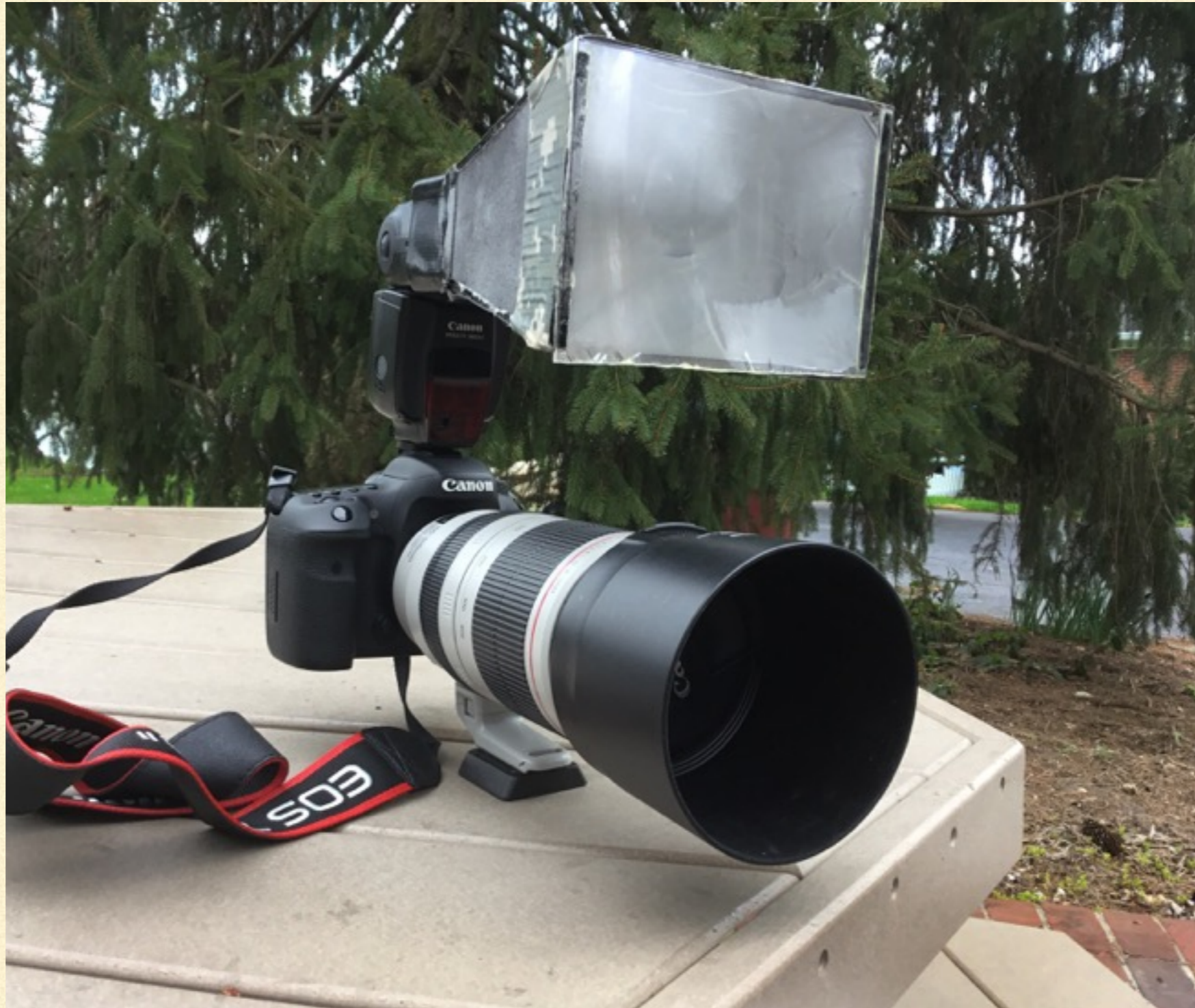
Canon 7D MkII, Canon Speedlite 580 EXII, Canon 100-400 lens, Home made flash extender
